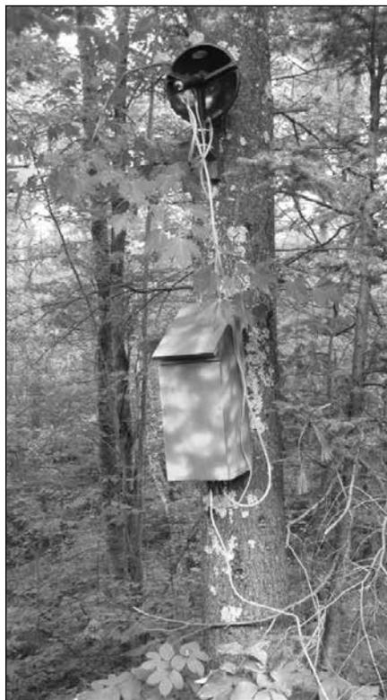
**Figure 2.** A howl box unit consisting of an outdoor speaker and parabolic microphone for recording.
